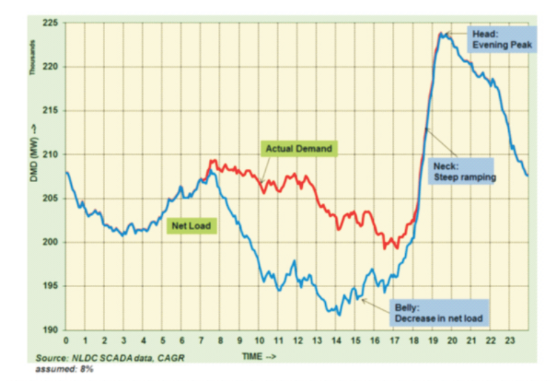
Fig. 7.1: Expected All India Net Load Curve With 20 GW of Solar Generation
