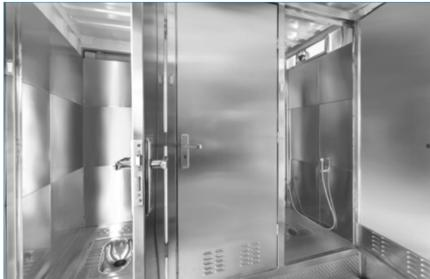
"Stainless steel modular toilets provide an appropriate solution for solving the problem of durability. In terms of structural strength, product life, maintenance, hygiene, eco-friendliness, and scrap value, stainless steel toilets have proved to be better than fibre, mild steel or brick-and-mortar toiles."
