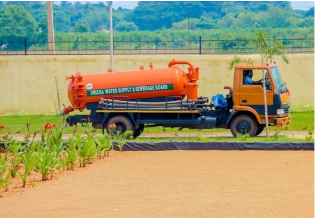
Desludging trucks for emptying on-site systems and conveying septage to treatment facility
